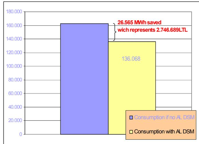
Presuming 88 % average efficiency and gas as the main fuel, estimated savings under AL DSM component reached more that 30,000 MWh of fuel and more that 6,000 tons of CO<sub>2</sub> during the life of the Project.
