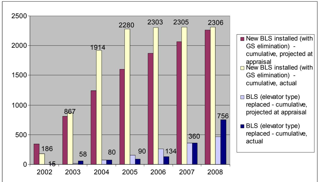
As a result of installation of new BLS, more that 157 km of hot water network was eliminated. Investments into replacement of BLS and modernization of network reduced losses in the district heating networks from 21 % (2002) till 13.7 % (2008). Since the completion of BLS program in 2006, so called “commercial losses” (heat wasted for heating “lost” cold water) have disappeared (see table No. 1).
